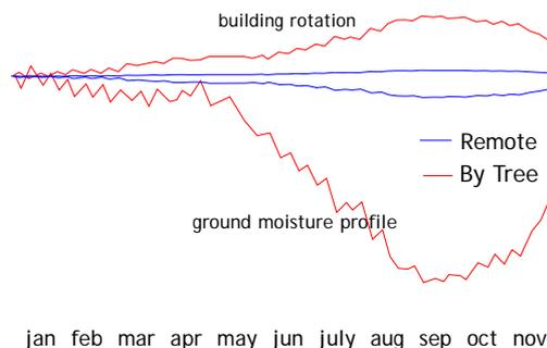
Instead of sinking boreholes, retrieving soils, testing them, monitoring and then asking the arborist if the tree is influencing the soil, The Clay Research Group have developed a combined and remote monitoring station, taking real time measurements of building and moisture movement - at the same time.
