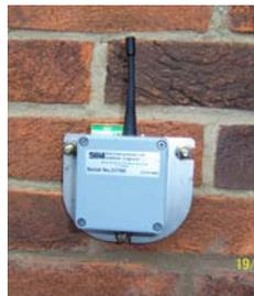
And then we add the tilt sensors. Measuring fine rotational movements and producing high value graphs taking readings every hour. We should start to see changes related to root activity in a few months time.
